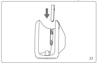
3) Slide the remote controller vertically down into the remote controller bracket ( $Fig.\ 24$ ).
