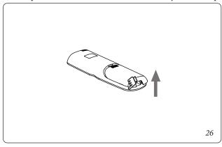
3) Take out the old batteries. Install two new AAA batteries according to the positive and negative polarities indicated (Fig. 27). Close the battery cover.
