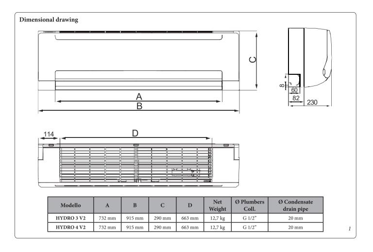
If the fan coil is to be installed on a metal part of the building, it needs to be electrically isolated in compliance with the applicable regulations on electrical appliances.
