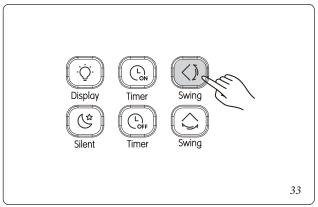
2) When the vertical swing is on, press (()) to turn off this function.
