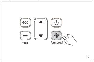
1)3 speeds: the fan speed will be adjusted in turn as shown below:
