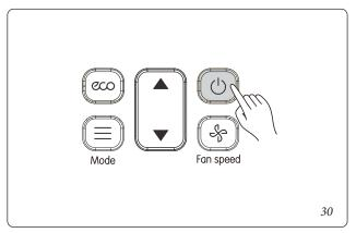
2)Press ((0)) again to stop the operation of the indoor unit. When the unit is off, the modes are visible on the display.
