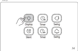
2)When the display of the indoor unit lights up, press to turn off the light.
