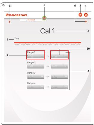
Pressing the button "Definition of interval start time" (Ref. 9, Fig. 26) or "Definition of interval end time" (Ref. 10, Fig 26) allows you to access the screen where you may define the start time ON and end time OFF using the "+" and "-" buttons.
