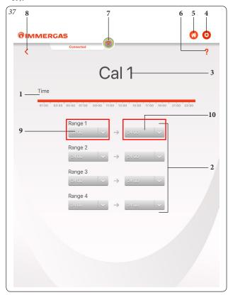
Pressing the button "Definition of interval start time" (Ref. 9, Fig. 37) or "Definition of interval end time" (Ref. 10, Fig. 37) allows you to access the screen where you may define the start time ON and end time OFF using the "+" and "-" buttons (Fig. 38).
