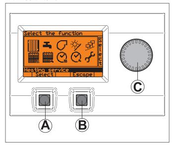
The control unit has a large display, two buttons (A and B) and a knob C.
