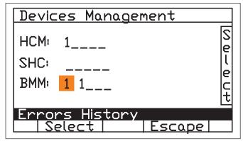
The display shows the devices in the system (- = not present/1-8 = progressive number of the detected device
