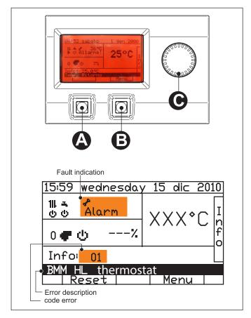
When the boiler detects a fault, the alarm symbol is displayed on the screen together with the relative error code and description.
