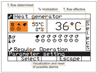
The highlighted part shows the operating status of the services (Central heating/DHW) and the generator:
