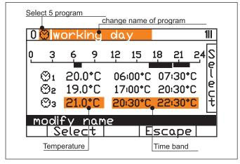
5 various "specific days" can be set and renamed (e.g. weekday, holiday, part time, etc.), and each one can have max of 3 request bands at 3 different temperatures ("room" for the Central heating menu or "storage tank" for the DHW menu).
