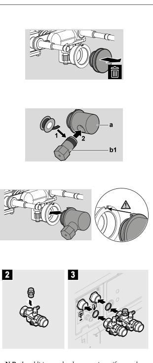
**N.B.:** In addition to the thermostatic antifreeze valve, a vacuum breaker valve is also supplied, which must be installed on the heat pump delivery valve (MHT) by removing the cap present.
