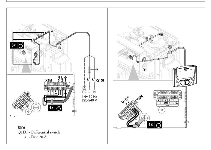
**Features of the outdoor unit connection.** The outdoor unit power cable (not standard supplied) must be suitable for outdoor installation and must have at least a flexible polychloroprene sheath (code IEC:60245 IEC 57 / CENELEC:H05RN-F).
