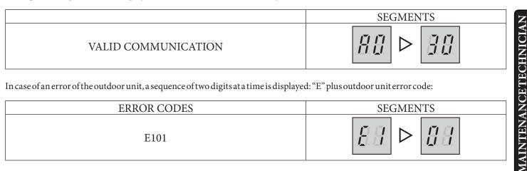
In case of an error of the outdoor unit, a sequence of two digits at a time is displayed: "E" plus outdoor unit error code:
