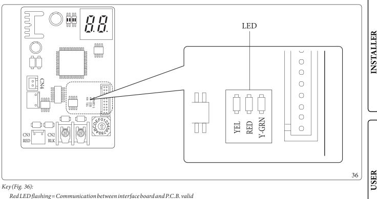
$Green \, LED \, flashing = Communication \, between \, interface \, board \, and \, outdoor \, unit \, valid$ Yellow LED = Not Used
