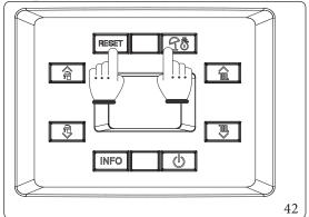
Press and hold buttons "RESET" and "T" for more than 5 seconds.
