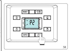
The first digit of the central indicator ( $\{\{\}\}\}$ ) shows the family of the parameter. The second digit shows the parameter number.
