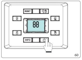
Press the mode of operation button "0" for more than 1 second to store the parameter value; confirmation is given by the word "H" which appears for 2 seconds.
