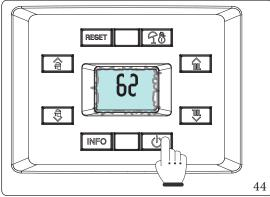
Press the "(1)" key to activate calibration. Once activated, the complete calibration function has four phases:
