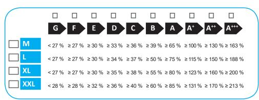
Water heating energy efficiency class in colder and hotter climate conditions
