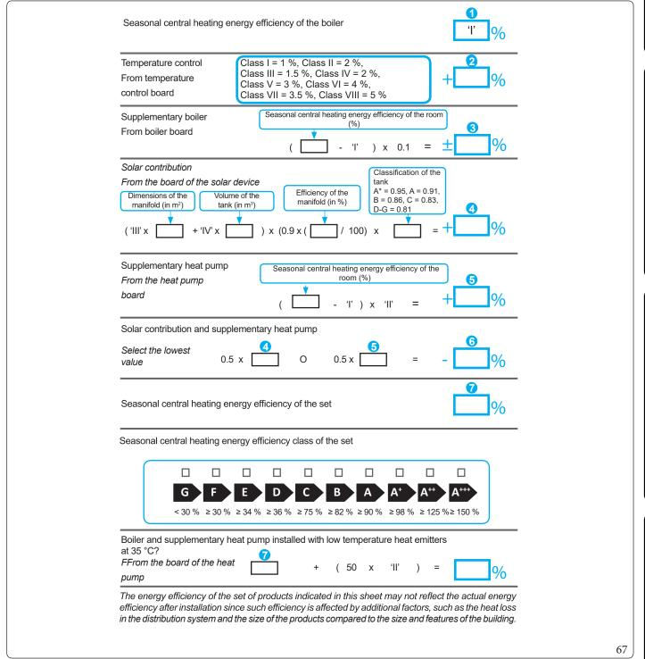
Parameters for filling in the assembly chart
