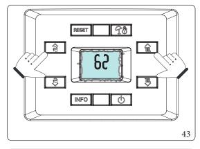
The display will show two dashes "--" flashing. Now enter the password "62" to activate the complete calibration (enter the first digit by pressing the 1-2 buttons
