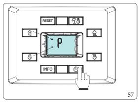
Once in the menu, you can cyclically scroll the submenus by pressing the D.H.W. buttons "  $\stackrel{•}{\triangleq} \stackrel{•}{\circlearrowleft}$ ", to access the menu press the button "  $\stackrel{•}{\textcircled{\scriptsize 0}}$ ".
