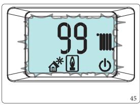
Only after the "[a]" symbol flashes is it possible to change the CO<sub>2</sub> value (Par. 3.10) or switch to the next heat output parameter by pressing the "U" button.
