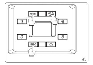
The function is activated from boiler in "off" by pressing and holding the "RESET", "INFO" and "To" buttons for more than 5 seconds.
