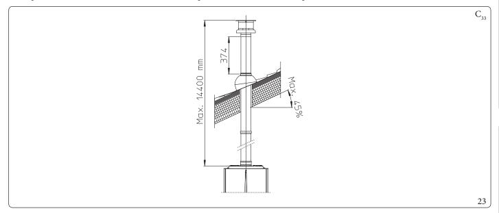
To install the kit Ø 80/125 one must use the flanged adapter kit in order to install the flue system Ø 80/125.
