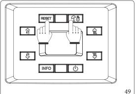
Press and hold buttons "RESET" and "To" for more than 5 seconds.
