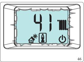
Only after the " Tymbol flashes is it possible to change the CO<sub>2</sub> value (Par. 3.10) or switch to the next heat output parameter by pressing the " button.
