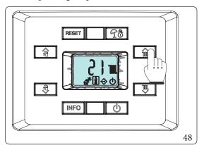
To increase the combustion setting, press the button  $5(\widehat{\mathbb{Q}})$ , to decrease it, press the button  $6(\widehat{\mathbb{Q}})$ . As the combustion setting increases, the  $CO_2$  value decreases and vice-versa.
