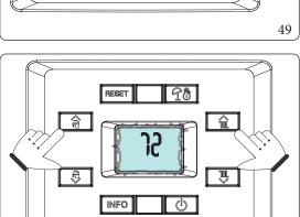
The display will show two dashes "--" flashing. Now enter the password "72" to activate fast calibration.
