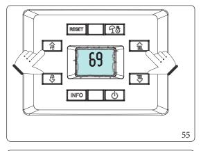
Now enter the password "69" to access the parameter menu. To enter the first digit, use the buttons to adjust the DHW " 会 ® "; to enter the second digit, use the buttons to adjust the central heating temperature " 1 3".
