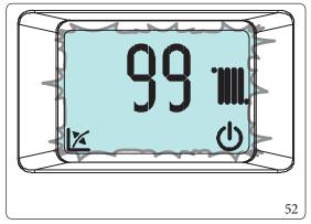
At this stage the display features flashing icons: "" and " 2" and the operating temperature is displayed, alternated with the current operating heat output.
