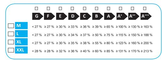
Water heating energy efficiency class in colder and hotter climate conditions
