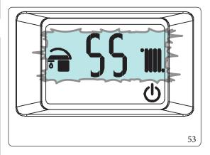
To activate the function, press the buttons "RESET" and "\(\bigcup\)" simultaneously until function activation, which is displayed by indicating the fan operation speed (in hundreds of revs) and ignition of the flashing "\(\bigcup\)" and "\(\bigcup\)" symbols.
