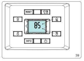
Its value can be adjusted by using the central heating temperature adjustment buttons "  $\widehat{\mathbb{Q}}$   $\mathbb{Q}$ ".
