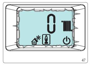
Only after the " $\P$ " symbol flashes is it possible to change the  $CO_2$  value (Par. 3.10) or switch to the calibration self-check phase by pressing the " $\P$ " button.
