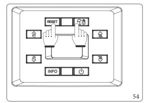
To access the programming phase, press and hold the buttons "RESET" and " Th" for more than 5 seconds, the display shows two dashes "--" flashing.
