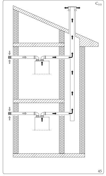
This configuration (allowed only with the approved original flue, including the specific non-return valve), makes it possible to suck the air outside the home or directly from the shaft where the flue gas exhaust is present and the evacuation of the flue gas itself inside a collective flue.
