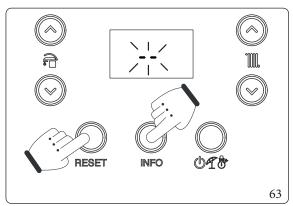
To access the programming phase, press and hold the buttons "RESET" and " INFO" for more than 5 seconds; the display shows two dashes "--" flashing and you must enter the password ( $^{\square}$ ) to access the programming menus.
