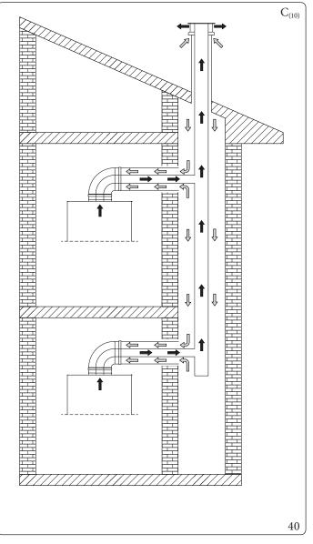
Installation in  $C_{(10)}$  configuration of an Immergas appliance (only permitted with approved original flue, including the specific non-return valve), makes it possible to intake combustion air directly from the shaft where the flue gas exhaust is present in the collective flue.
