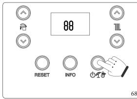
Press the mode of operation button "MT" for more than 1 second to store the parameter value; confirmation is given by the word " $\mathbf{88}$ " which appears for 2 seconds.
