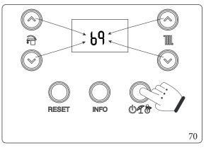
To enter the first digit use the buttons to adjust the DHW , to enter the second digit use the buttons to adjust the central heating temperature . To confirm the password and access the menu, press the operating mode button " \( \mathbb{O} \) \( \mathbb{O} \) "
