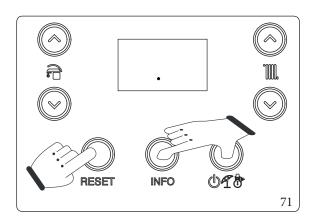
The function is activated from boiler in "off" by pressing and holding the " RESET", "INFO" and "Off" buttons for more than 5 seconds.
