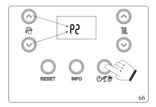
The first digit of the central indicator (Fig. 58) shows the family of the parameter, while the second digit shows its number.
