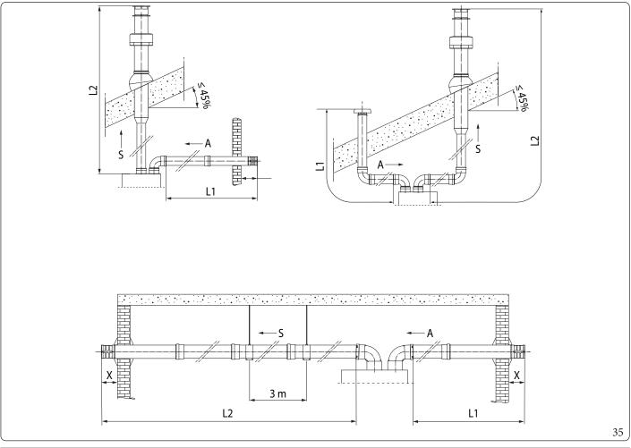
To calculate the equivalent length of the flue (L), simply add, for each component you intend to use, the corresponding value indicated in the column "Length equivalent to m of pipe" in the table in par. 1.15, and check that the resulting sum is equal to or less than the maximum length (L max) indicated in par. 1.16. (L  $\leq$  L max).
