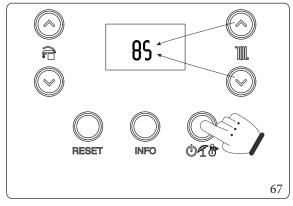
Pressing the mode of operation button "Off" displays the value of the selected parameter and by pressing the buttons to adjust the central heating temperature "o" you can adjust its value.
