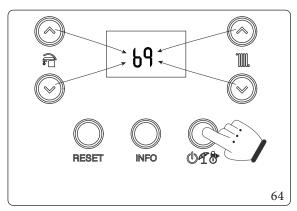
To enter the first digit use the buttons to adjust the DHW ., to enter the second digit use the buttons to adjust the central heating temperature ...
