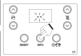
Press and hold the "INFO" button for more than 5 seconds. The display will show two dashes "--" flashing. Now enter the password ( $\P$ ) to access the programming menus.
