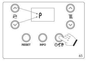
Once in the menu, you can cyclically scroll the four submenus (P, t, A, S) by pressing the DHW buttons " $^{\textcircled{a}}$ ", to access the menu press the button " $^{\textcircled{a}}$ ".
