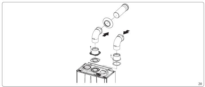
In case of installation  $C_{(10)3}/C_{(12)3}$  the flue gas non-return valve must be installed and ONLY the vertical outlet can be installed in the recessed frame.
