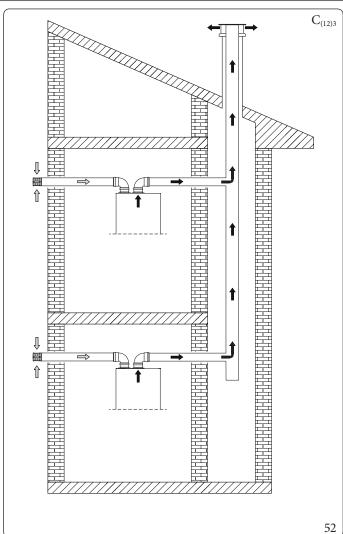
This configuration (allowed only with the approved original flue, including the specific non-return valve), makes it possible to suck the air outside the home or directly from the shaft where the flue gas exhaust is present and the evacuation of the flue gas itself inside a collective flue.
