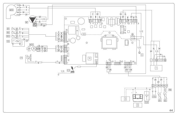
$Comando\ Amico\ Remoto\ v2: the\ boiler\ is\ prepared\ for\ the\ application\ of\ the\ Comando\ Amico\ Remoto\ remote\ control\ v2\ (CAR^{v2}), which\ must$ be connected to clamps 41 and 44/40 of the terminal board (located in the boiler control panel) respecting the polarity and eliminating link X40.
