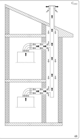
Installation in  $C_{(10)3}$  configuration of an Immergas appliance (only permitted with type-approved original flue, including the specific non-return valve), makes it possible to extract combustion air directly from the shaft where the flue gas exhaust is present in the collective flue.
