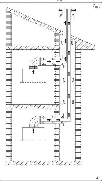
Installation in  $C_{(15)3}$  configuration of an Immergas appliance, makes it possible to extract combustion air directly from the shaft where the flue gas exhaust is present in the dedicated flue.
