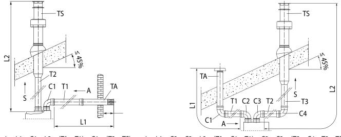
L = L1 + C1 + L2 = (TA + T1) + C1 + (T2 + TS)L = L1 + C2 + C3 + L2 = (TA + C1 + T1) + C2 + C3 + (T2 + C4 + T3 + TS)
