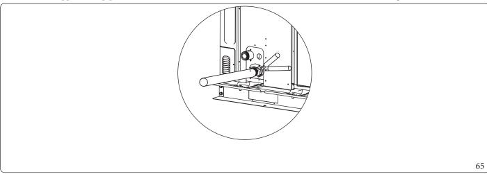
The unit must be used in a closed water system only. The application in an open water circuit could cause excessive corrosion to the water pipes:
