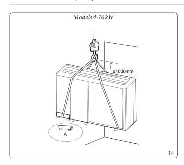
The hook and the centre of gravity of the unit must be on a vertical line to avoid an improper inclination.
