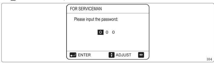
Press to navigate and press to adjust the numerical value. Press . The password is 234, the following pages will be displayed after having entered the password:
