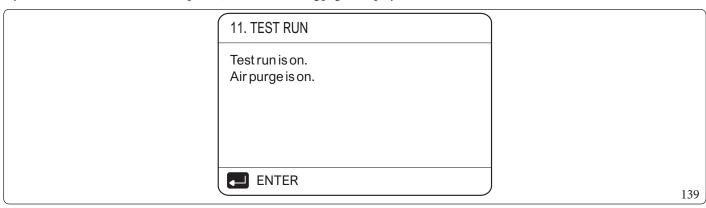
When in the air purge mode, SV1 opens, SV2 closes. 60 seconds later, the pump in the unit (PUMP\_I) will run for 10 minutes during which the flow switch will not work. After the pump stops, SV1 closes and SV2 opens. 60 seconds after both "PUMP\_I" and "PUMP\_O" will run until they receive the next command.
