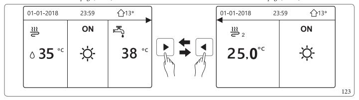
In this case, the setting value of zone 1 is T1S, the setting value of zone 2 is T1S2 (the corresponding T1S2 is calculated based on the climatic curves).
