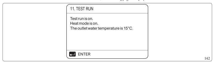
During execution of the "HEATING" test, the default temperature of the outlet water is 35°C. The IBH switches on after the compressor has been operating for 10 minutes. After 3 minutes of operation of the IBH, the IBH switches off, the heat pump runs until the water temperature increases to a certain value or another command is received. Selecting "11.6 DHW MODE RUNNING" displays the following page:
