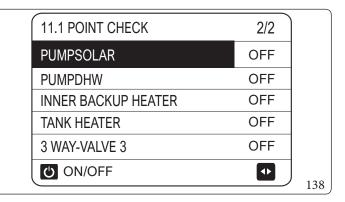
Press  $\bigvee \Delta$  to scroll to the components you want to check and press  $\bigcup$ . For example, when the 3-way valve is selected and  $\bigcup$  is pressed, if the 3-way valve is open/closed, then operation of the 3-way valve is normal, as are the other components.
