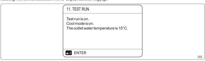
$During \, operation \, of the \, ``COOL \, MODE" \, test, the \, default \, temperature \, of the \, outlet \, water \, is \, 7°C. \, The \, unit \, will \, operate \, until \, the \, water \, temperature \, drops to a \, certain \, value \, or \, a \, subsequent \, command \, is \, received.$
