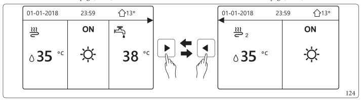
In this case, the setting value of zone 1 is T1S, the setting value of zone 2 is T1S2.
