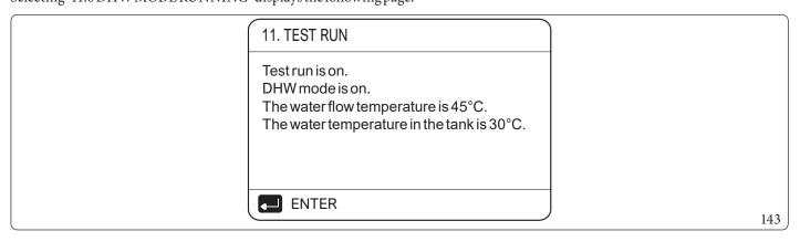
During execution of the DHW MODE test, the default temperature of the domestic hot water is 55°C. The TBH (DHW tank booster heater) switches on after the compressor has been operating for 10 minutes. The TBH will switch off 3 minutes later, the heat pump will run until the water temperature increases to a certain value or another command is received.
