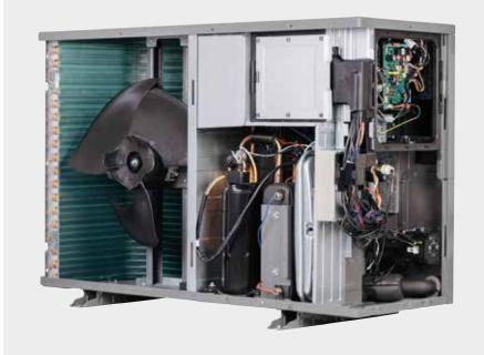
**Refrigerant circuit** equipped with inverter compressor (Rotary for versions 5–8 and Scroll for versions 12–16), electronic lamination valve, 4-way reversing valve, high and low pressure switches
