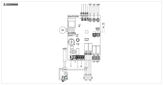
Rigid or flexible wires with a 0.2 to 1.5 mm² cross-section (0.75 mm² if two wires are connected to the same terminal block) can be inserted in the 4 spring-loaded terminal blocks (ref. A) for connection of the wall-mounted controller 3.029897/3.029898. If the wires have wire end ferrules with a plastic collar, the maximum cross-section
